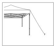
\*FRAME MUST BE SECURED DOWN TO PREVENT WIND FROM LIFTING TENT AND CAUSING DAMAGE. NOT SECURING TENT PROPERLY VOIDS THE WARRANTY.
